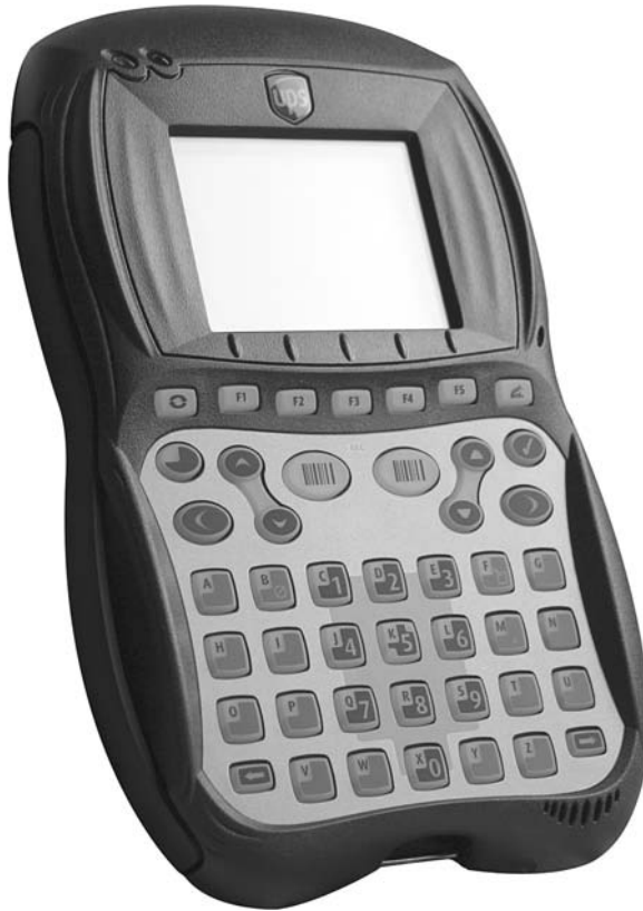
Figure 3.2 UPS Diad IV targeted work device for drivers. Image downloaded from http://pressroom.ups.com
