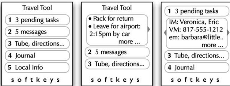
Figure 10.1 Fisheye portal design for a scroll and select device. The left pane shows no item highlighted, and all portlets minimized. The center pane shows the result of scrolling down one click, highlighting the first portlet and expanding it. The right pane shows the result of scrolling down a second click, with the first portlet minimized again and the second portlet expanded.
